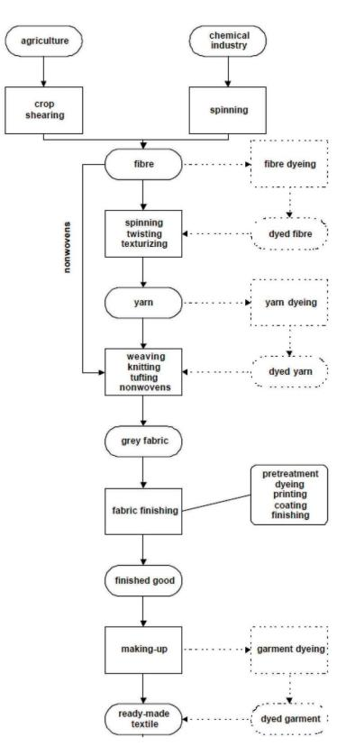
*Figure 3 : A simplified schematic picture of the textile manufacturing process (KemI, 2013)*
