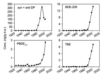
Figure 10 Concentration of BTBPE (TBE) and other brominated flame retardants in a sediment core from Lake Ontario as a function of year of deposition. Figure from Qiu *et al.* (2007).
