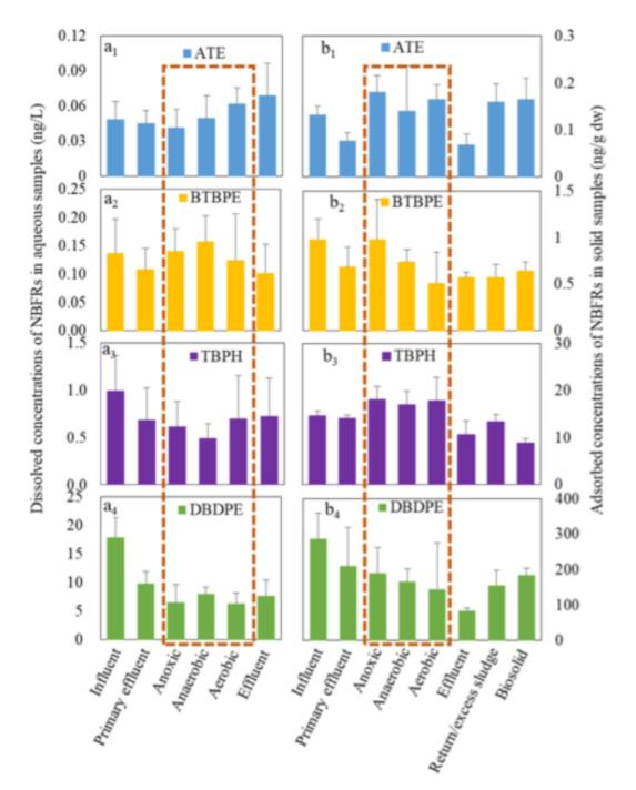
Figure 9 BTBPE and other NBFR concentrations measured in the a) wastewater (dissolved, ng/L) and b) biosolid samples (adsorbed, ng/g dw) from different treatment units in the WWTP in the study by Wang *et al.* 2020. Figure taken from Wang *et al.* (2020).
