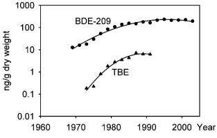
Figure 11 Concentration of BTBPE (TBE) and BDE-209 as a function of depth in the Lake Michigan sediment core. Figure from Hoh *et al.* (2005).
