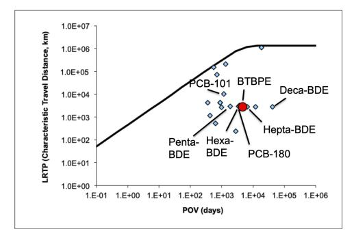
Figure 16 OECD LRTP-P<sub>ov</sub> tool plot comparing BTBPE (red dot) and benchmark POPs (grey diamonds) for CTD and  $P_{ov}$  (Wegmann *et al.* 2009). See Table 9 for input data used in the tool.
