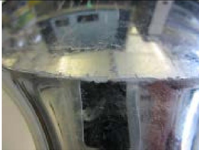
*Figure 1. Abrasive behaviour of tested part (after 3 months) coated with ePD. The performance is clearly not in line with industry standards. At the edges spalling of the coating is visible.*
