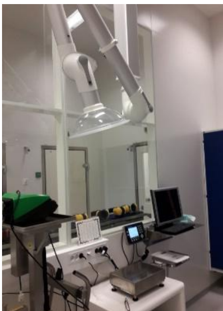
Image of extraction unit used during the dispensing/weighing of PFOB.
