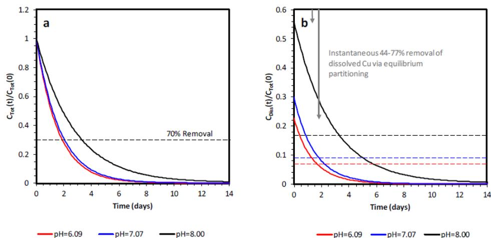
**Figure 3. a) Dissolved and b) total copper removal from the water column under different pH conditions for a DOC concentration of 15 mg/L. Copper speciation (including binding to POC) was calculated using WHAM V in TICKET-UWM. The initial total copper concentration in the water column,  $C_{Tot}(0)$ , was set at the pH-specific acute ERV (Table 2-1). The horizontal dashed line represents  $C(t)/C_{Tot}(0) = 0.3$  or 70% removal of copper.**
