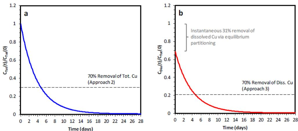
**Figure 1. a) Total and b) dissolved copper (Cu) removal from the water column using EUSES model parameters and the linear partitioning method. The initial total copper concentration in the water column,  $C_{Tot}(0)$ , is 35  $\mu\text{g/L}$ . The horizontal dashed lines represents a)  $C_{Tot}(t)/C_{Tot}(0) = 0.3$  (70% removal of total copper) and b)  $C_{Diss}(t)/C_{Diss}(0) = 0.3$  (70% removal of dissolved copper).**
