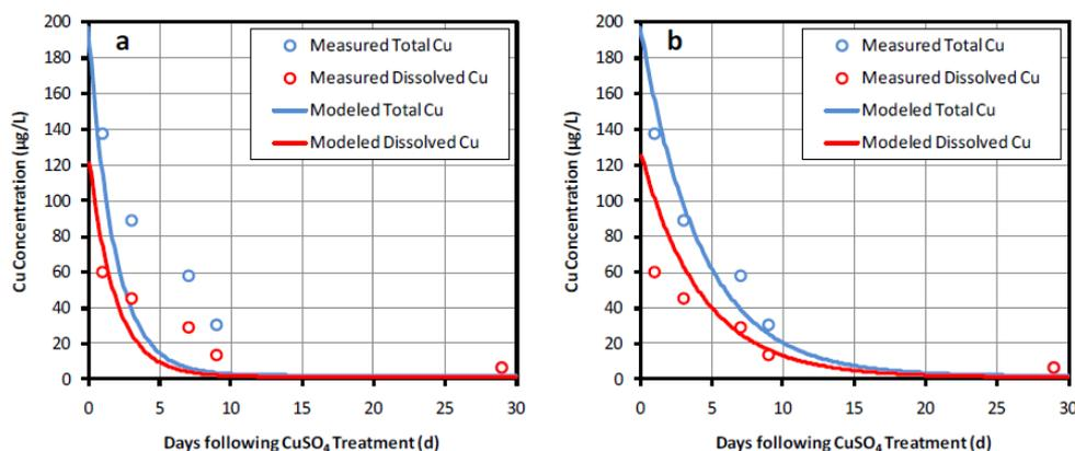
**Figure 10.** Comparison of TICKET-UWM output (lines) and measured data (points) for copper in the water column of the Saint Germain les Belles Reservoir: EUSES scenario. Model results are from a) the EUSES scenario (water column  $K_D$   $10^{4.48}$  L/kg; sediment  $K_D = 10^{4.39}$  L/kg, and settling velocity = 2.5 m/d) and b) the EUSES scenario with the settling velocity reduced to 1.02 m/d.
