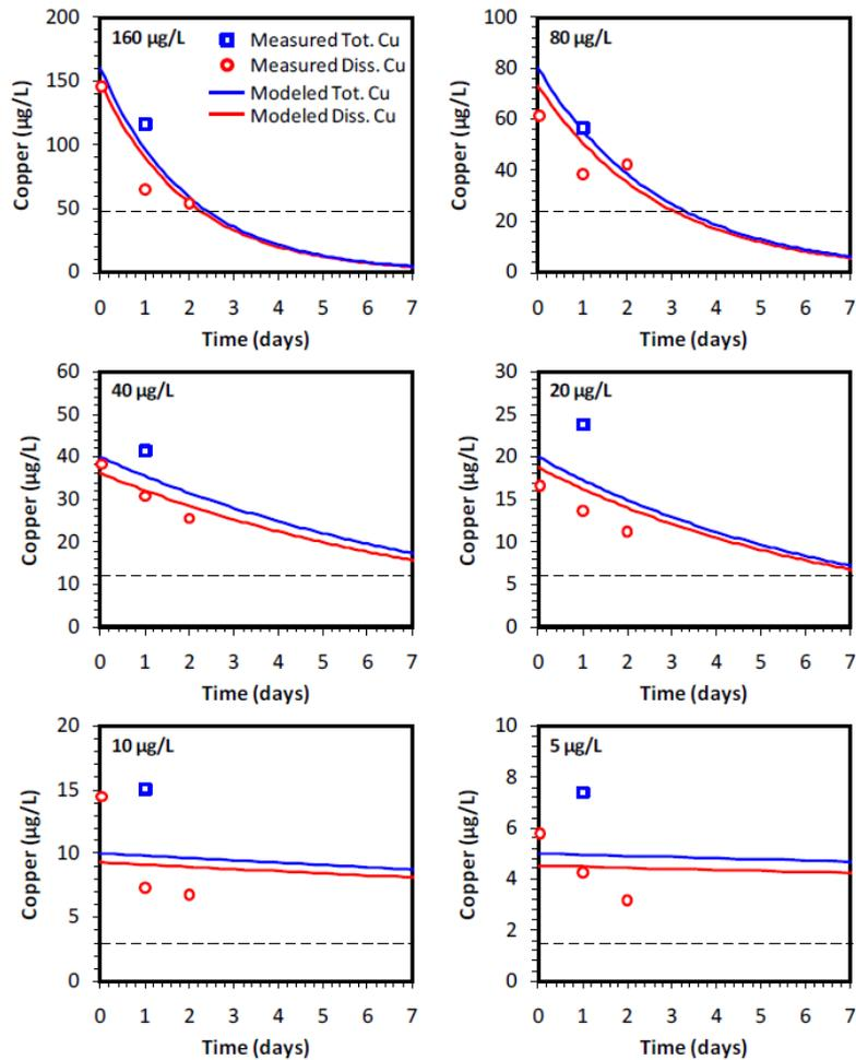
**Figure 14. Comparison of TICKET-UWM output (lines) to measured data (points) for total copper (blue squares and lines) and dissolved copper (red circles and lines) in the water column of the IME microcosms for the EUSES scenario with optimized settling velocities. The horizontal black dashed line denotes 70% dissolved copper removal relative to the nominal value.**
