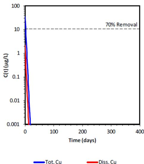
**Figure 8. TICKET-UWM simulations with water column isolated from the sediment (i.e., no feedback/remobilization) for initial total copper equal to 35 µg/L. The dashed line is at a concentration corresponding to 30% remaining (70% removal) based on the initial total concentration.**
