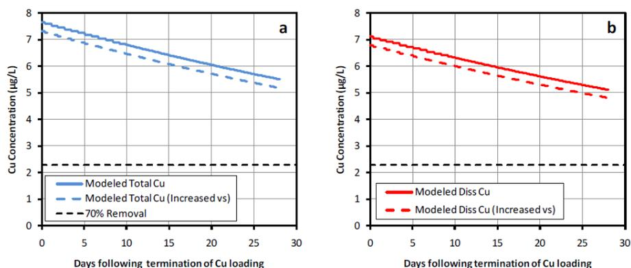
**Figure 13.** a) Total and b) dissolved copper TICKET-UWM results from post-loading simulations for the observed  $K_D$  and settling velocity scenario. Model simulations use the experimentally-estimated values for the water column  $K_D$  (104.12 L/kg) and settling velocity (0.2 m/d). The blue and red dashed lines refer to simulations with the settling velocity increased to 0.28 m/d. The horizontal black dashed line denotes 70% copper removal.
