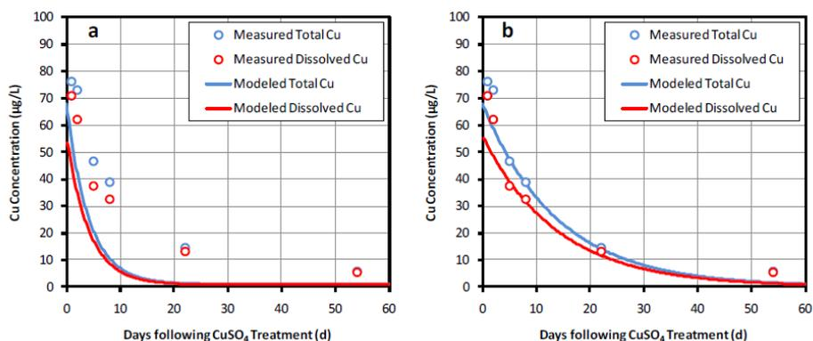
**Figure 9. Comparison of TICKET-UWM output (lines) and measured data (points) for copper in the water column of Lake Courtille: EUSES scenario. Model results are from a) the EUSES scenario (water column  $K_D$   $10^{4.48}$  L/kg; sediment  $K_D = 10^{4.39}$  L/kg, and settling velocity = 2.5 m/d) and b) the EUSES scenario with the settling velocity reduced to 0.70 m/d.**
