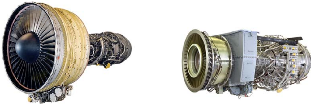
Figure 4. Left: CF6 Aircraft Engine. Right: Technology from the CF6 engine in generating power for the world’s largest hospital (The General Electric Company, 2014).
