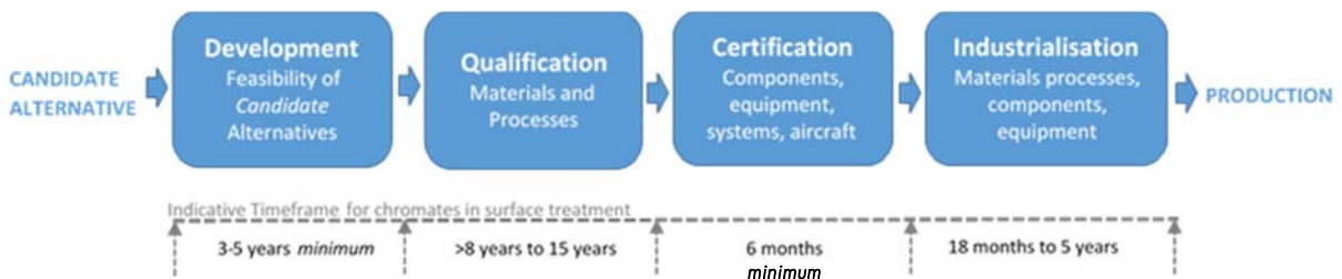
Figure 2: Illustration of the development, qualification, certification and industrialisation process required in the aerospace sector.
