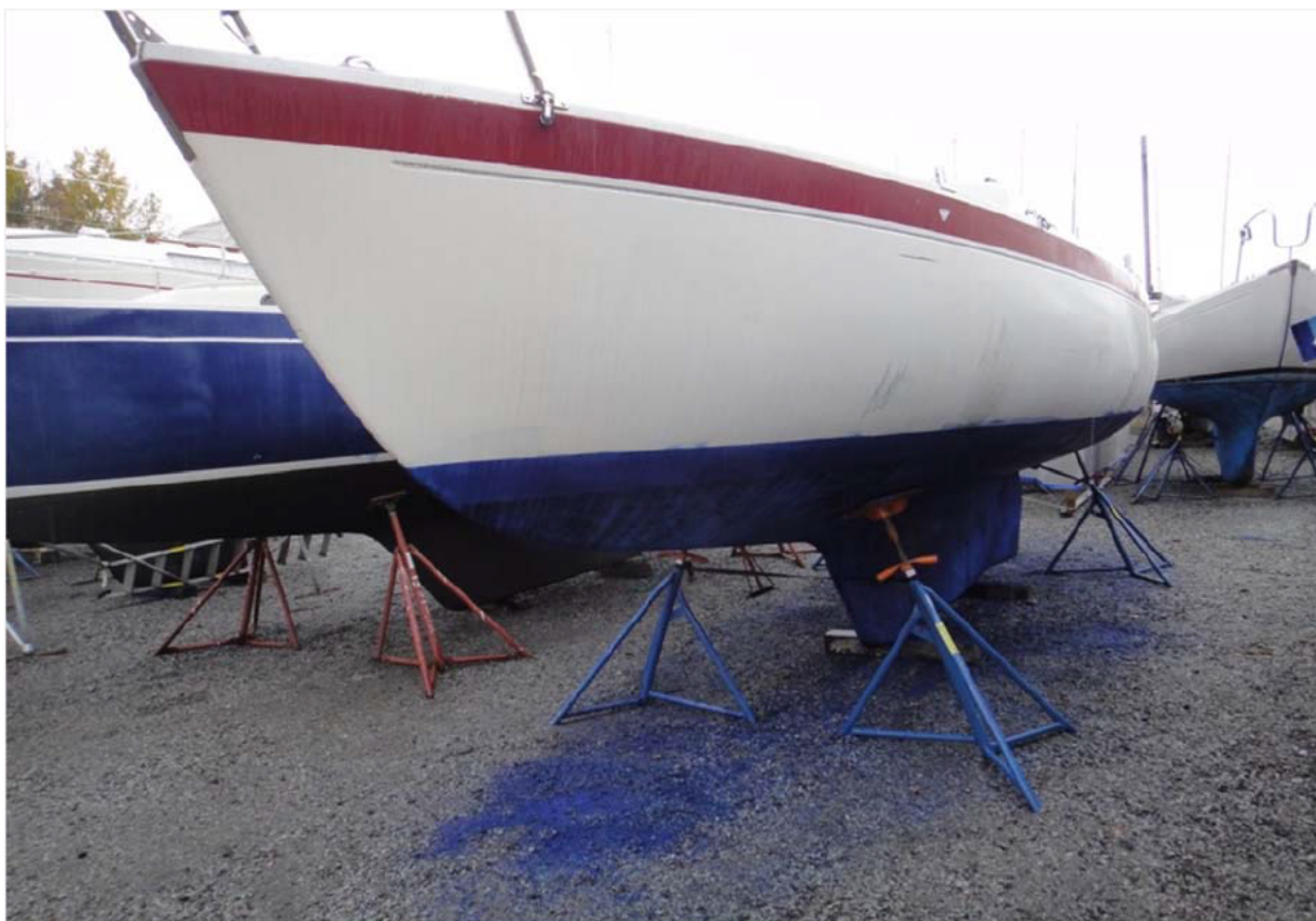
Figure 2.2.3.4. Emission of paint particles onto soil during maintenance and repair. (Photo by Britta Eklund, Stockholm University).
