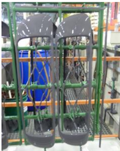
Figure 12: Electroless nickel coated ABS, intermediate step. Data source: FGK, 2014.
