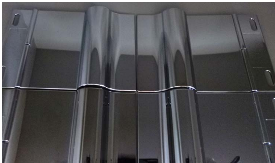
Figure 18: Pattern coated with different trivalent chromium based electrolytes showing the different shades of colour. Data source: BMW, 2014.
