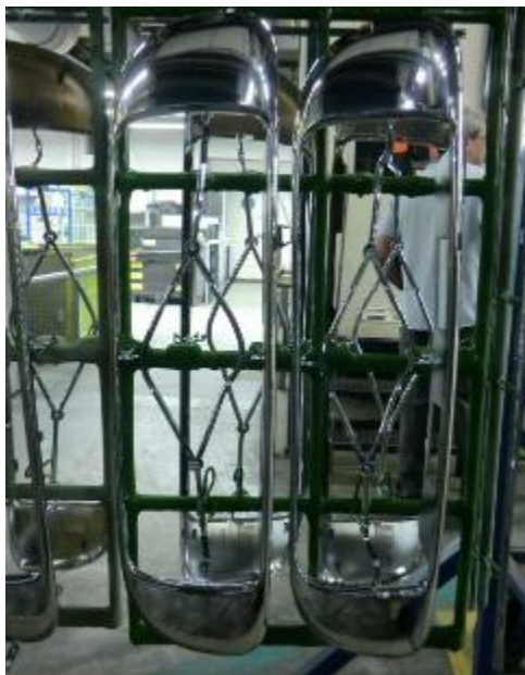
Figure 13: Metallic chrome coating from chromium trioxide based electroplating on ABS, final process step. Data source: FGK, 2014.
