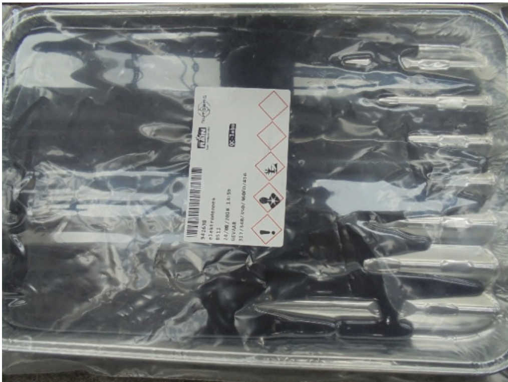
Figure: New pitch sampling container, closed, with pictograms
