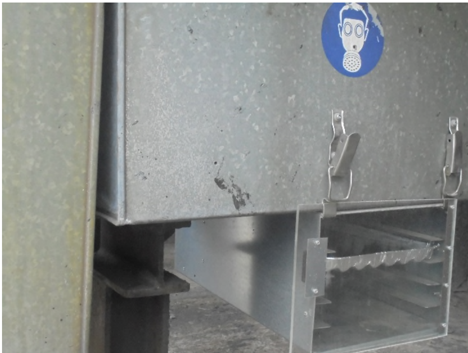
Figure: Fully closed pitch sampling box with sampling container (closed) with a sign indicating that a respiration mask needs to be worn when opening the sampling box
