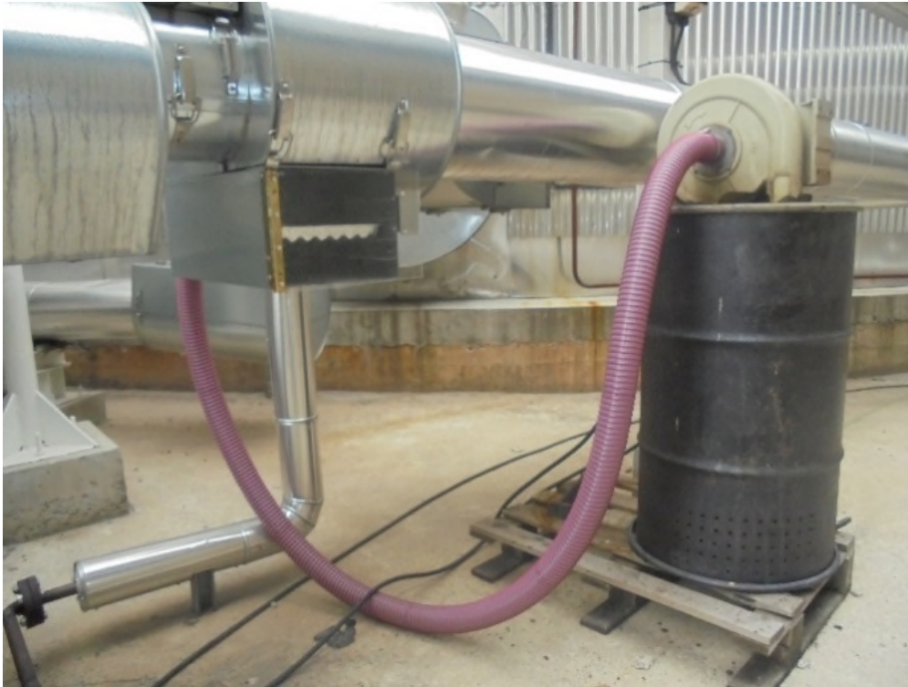
Figure: Fully closed pitch sampling box equipped with local ventilation and cleaning of the extracted air on an active carbon adsorbent
