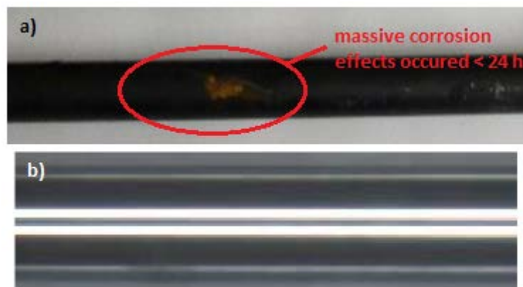
Figure 28: Direct comparison of a) case hardened piston rod b) Cr(VI) coated piston rod after salt spray test (DIN EN ISO 9227 NSS)
