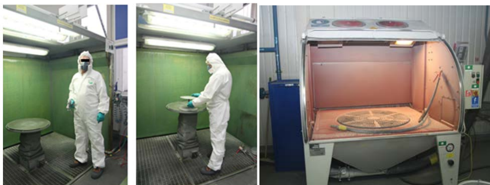
Fig. 3: Preparation of the coating process: Masking and sandblasting.
