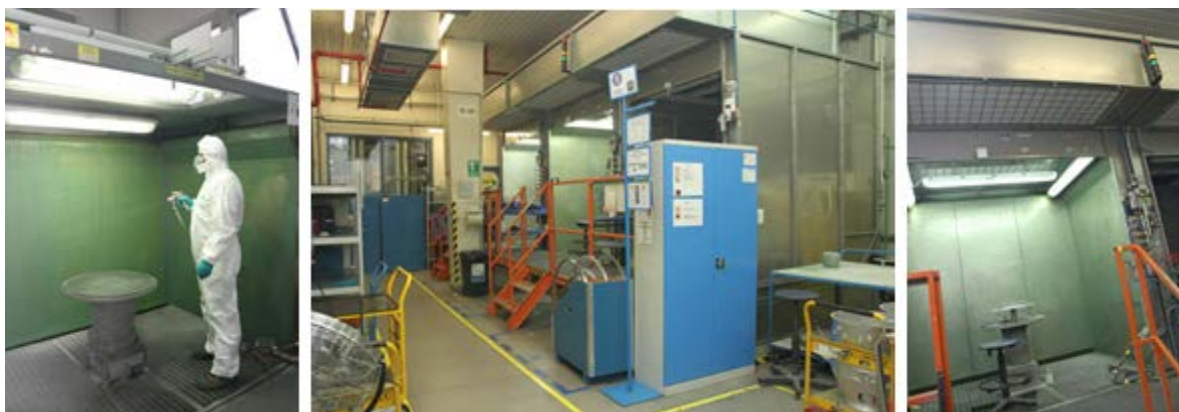
Fig. 4: Manual application of several coating layers in open paint booth.
