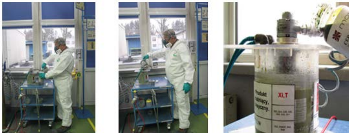
Fig. 2: Filling of the hand-paint gun.
