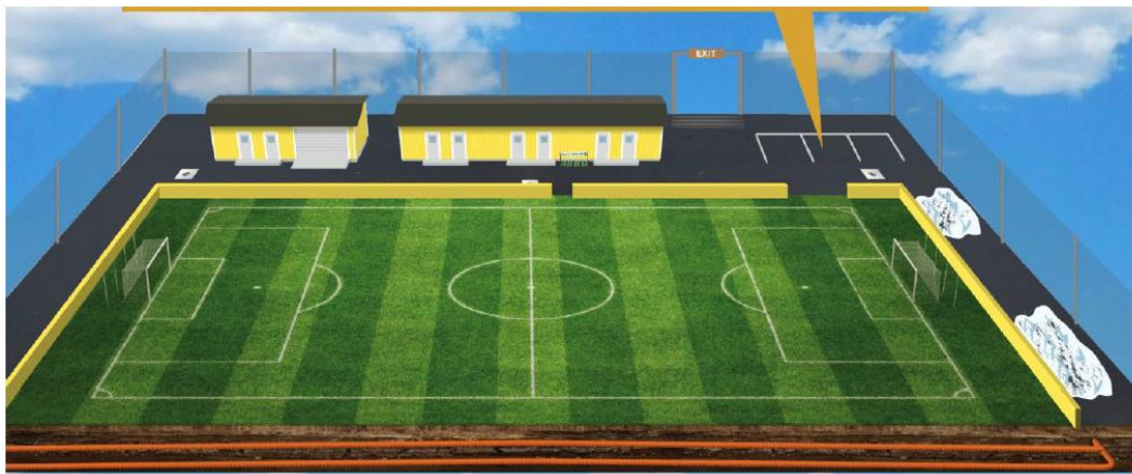
Figure 21: Example of a field with fences to avoid dispersion from visitors and a dedicated area for cleaning maintenance machinery. Source: ETRMA (2019).
