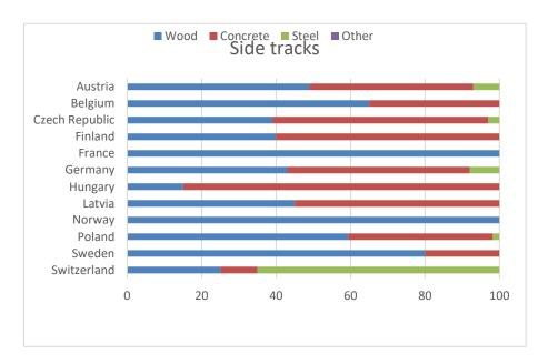
Figure B - 3: Use ratio between concrete and wooden sleepers in side tracks in European railways (figures for 2010, from UIC, 2013)
