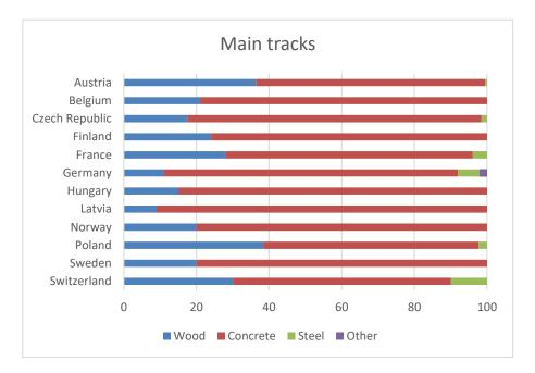
Figure B - 6: Use ratio between concrete and wooden sleepers in main tracks in European railways (figures for 2010, from UIC, 2013)
