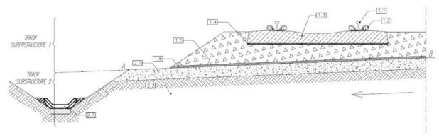
Figure B - 1: Components of a ballasted track system (from Zbiciak et al., 2017)
