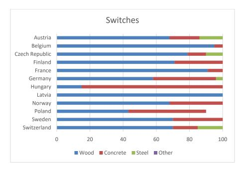
Figure B - 9: Use ratio between concrete and wooden sleepers in switches in European railways (figures for 2010, from UIC, 2013)
