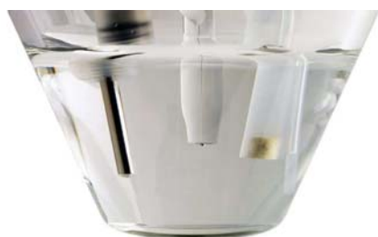
The Metrohm 3 electrode system. (the real physical diameter of the mercury drop is typically between 0.3 mm and 0.4 mm; the size is adjustable in certain narrow limits).
