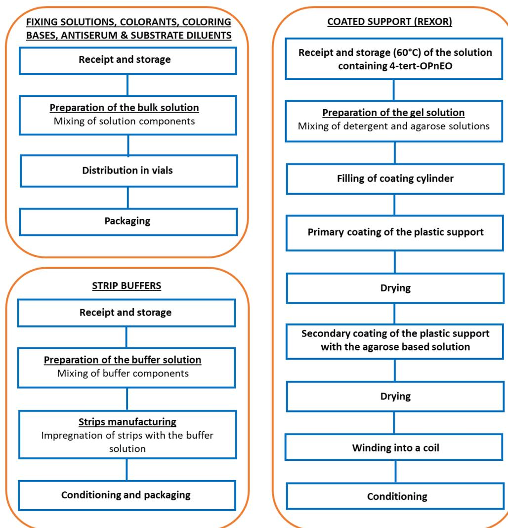
Figure 18. General production processes of reagents and additives solutions composing SEBIA kits and coated support supplied by REXOR
