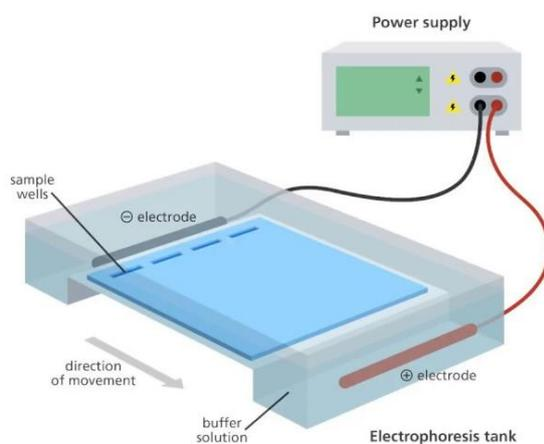
**Figure 4. Gel electrophoresis scheme**
