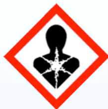
Serious Health hazard
