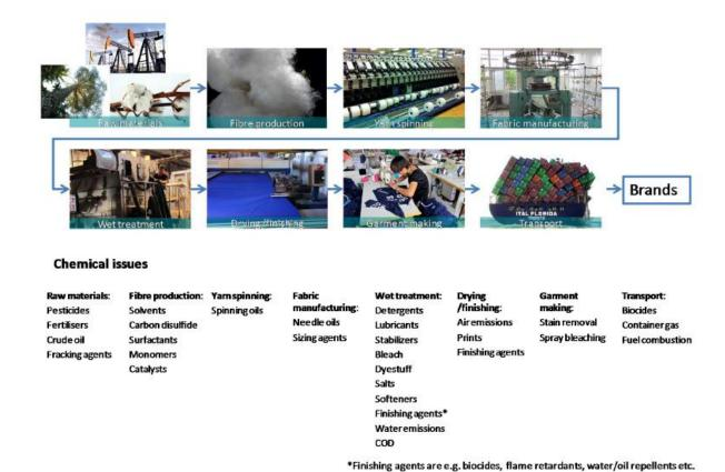
Figure 1. Overview of the textile production process and the types of chemicals used in the different steps (Roos, 2015) (© Swerea IVF)
