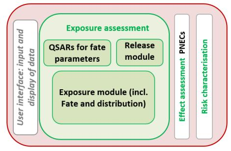
Figure 2: High-level description of the structure of EUSES
