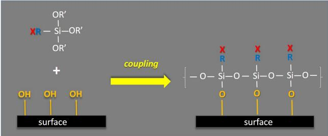
**Figure 2:** Schematic of an organosilane surface treating agent XR-Si-(OR')<sub>3</sub> and the chemistry it imparts to the surface of the particle after surface treatment.
