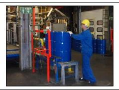
Loading of empty drums for automated filling
