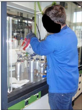
Task: filling small containers for further analysis in a laboratory setting. The labels are attached to the bottles once the transfer is completed.
