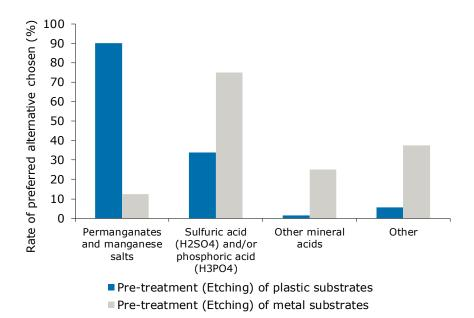
Figure 21: Preferred alternatives of the DUs for the substitution of CrO3 in the sub-uses "Pre-treatment (etching) of plastic substrates" and "Pre-treatment (etching) of metal substrates"
