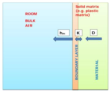
Figure 1. Illustration of the mechanisms driving releases from a solid matrix
