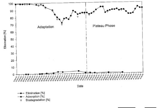
Figure A7\_1\_2\_1\_1-1: Elimination, biodegradation and adsorption of OIT of during adaptation and plateau phase
