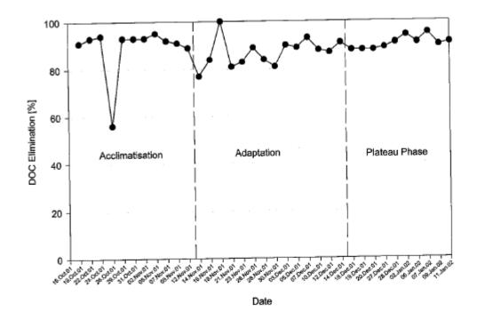
Figure A7\_1\_2\_1\_1-2: Elimination of DOC in the organic medium during the test
