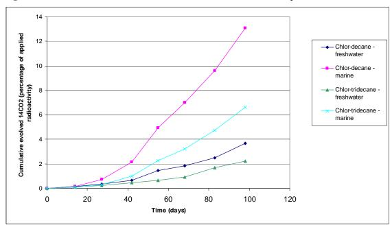
Figure 1 Mineralisation of <sup>14</sup>C-labelled short-chain chlorinated paraffins in aerobic sediments
