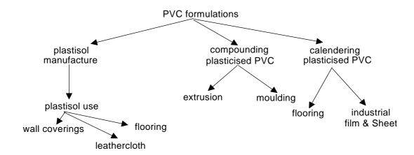
The exposure to MCCPs in the plasticisation of PVC is considered under the following headings: PVC plastisol manufacture, PVC plastisol use, calendering of plasticised PVC, compounding of plasticised PVC, and extrusion and moulding of plasticised PVC.
